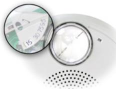
Genesis output levels are changed by simply opening the device and sliding the selectors to the desired settings. Settings remain visible through small windows on the device even after the cover is closed.
